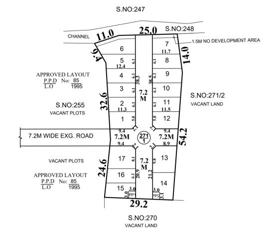
SITE EXTENT 1983 SQ.M (AS PER DOCUMENT) **ROAD AREA** 660 SQ.M PUBLIC PURPOSE PROVIDED (1%) 18 **SQ.M** PP-1 HANDED OVER TO THE LOCAL BODY: 9.0 SQ.M PP-2 HANDED OVER TO THE TANGEDCO : 9.0 SQ.M NO.OF PLOTS 17 Nos. NOTE: 1. SPLAY - 1.5M x 1.5M 2. MEASUREMENTS ARE INDICATED EXCLUDING SPLAY DIMENSIONS 3. ROAD AREA PUBLIC PURPOSE-1
